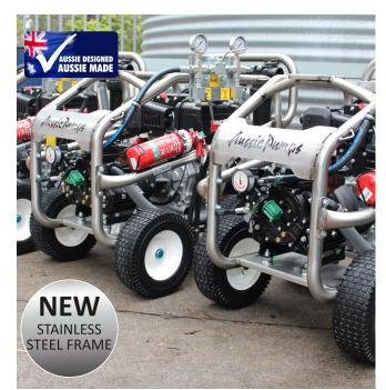
This range of hydrostatic testers consist of reliable Udor diaphragm pumps driven by petrol or diesel engines.
